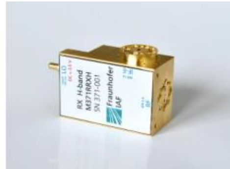
Fig. 2: Receiver block diagram (left) and the corresponding module (right).
