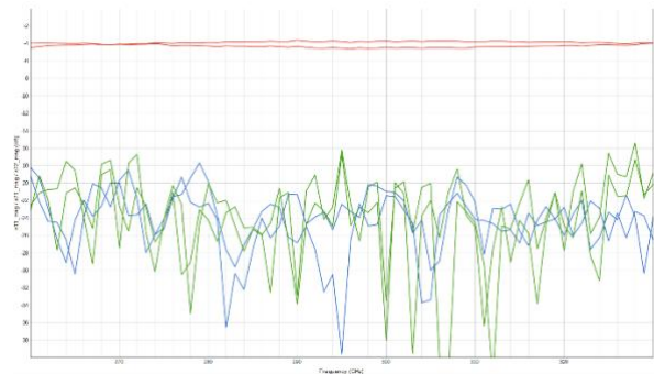
Figure 8: Employed combiner for PoC2 with mechanical drawing and measured S-parameters.
